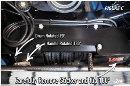
11.) Carefully rotate the cables so they are facing up through the notch and route them across the winch plate. The three holes on the back edge of the plate are for zip ties to attach the cables to the plate and secure them neatly. They will be aimed towards the passenger side of the Bronco at this time. IMPORTANT: Be sure that no cable ends at the winch are contacting each other and the rubber isolator boots are used after all nuts are tight.
