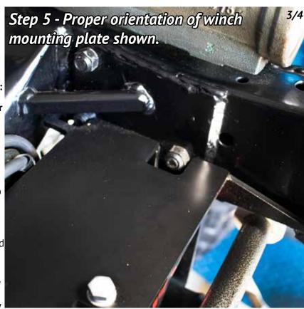
14.) Carefully reach into the frame rails and install the 4 bolts into the front of the mount and thread on the nuts and washers.
