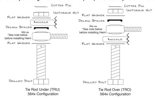
\*Note: Delrin spacers can bind the heim steering and make it touchy on the road, if the tops of the knuckles are not flat and the heim stud hole is not 100% perpendicular with the knuckle mounting face.
